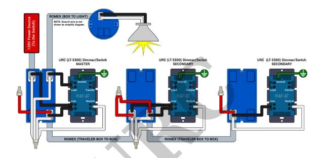
LT-3300: 4-Way Wiring Diagram. Line/Load in Separate Boxes:
