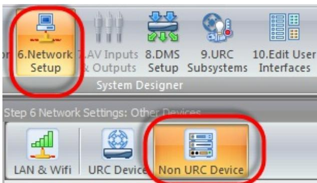
2. The window displays a list of the **Non URC network devices**. For the Master System
