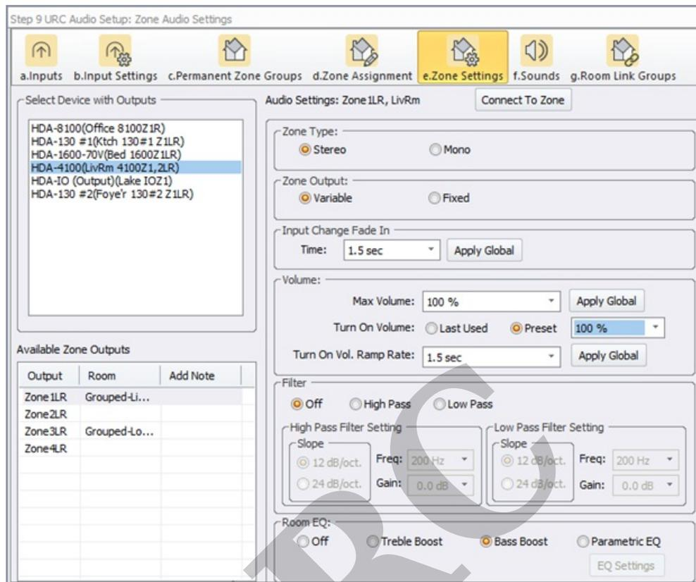
If a "Full Range" Line Level audio output from the Preampfier Output is desired, set the "Max Volume" parameter to "100%" and the "Turn On Volume" to "Preset – 100%".
