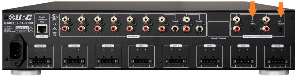
HDA-IO rear panel showing the 12V CTRL (output) location:
