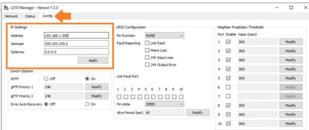
7. In the “Config” tab, set the following settings in the “Switch Options” section:
