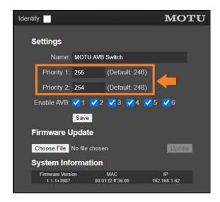
4. Verify that all six ports on the Motu AVB Switch are "checked" to enable AVB:
